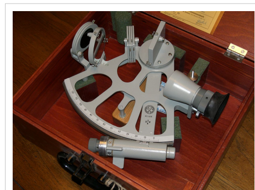
Sextants are used to measure the angle of the sun or stars with respect to the horizon. Using trigonometry and a marine chronometer, the position of the ship can be determined from such measurements.
