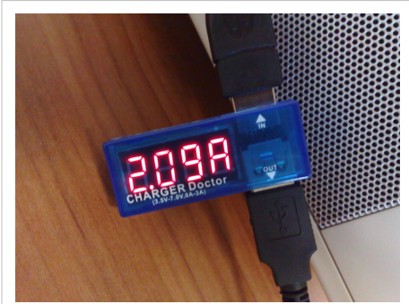
Small gadget providing voltage and current readouts for devices charged over USB.
