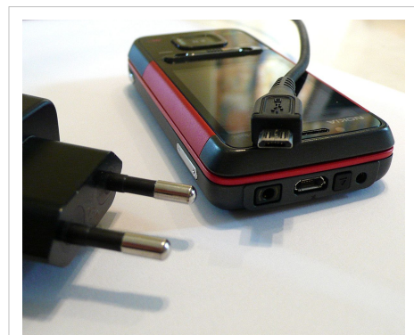
The Micro-USB interface is commonly found on chargers for mobile phones
