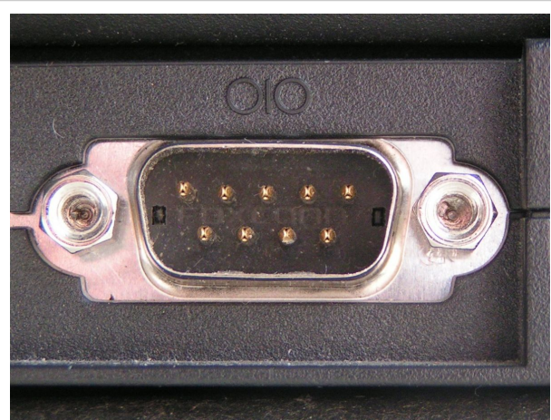
A male DE-9 connector used for a serial port on an IBM PC compatible computer along with the serial port symbol. (Pinout)
