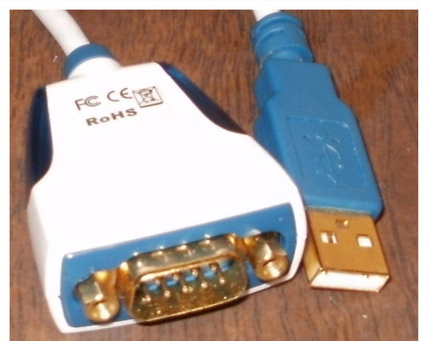
A converter from USB to an RS-232 compatible serial port; more than a physical transition, it requires a driver in the host system software and a built-in processor to emulate the functions of the IBM XT compatible serial port hardware.
