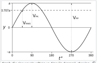
Graph of a sine wave's voltage vs. time (in degrees), showing <sup>□</sup> RMS, peak (PK), and peak-to-peak (PP) voltages.
