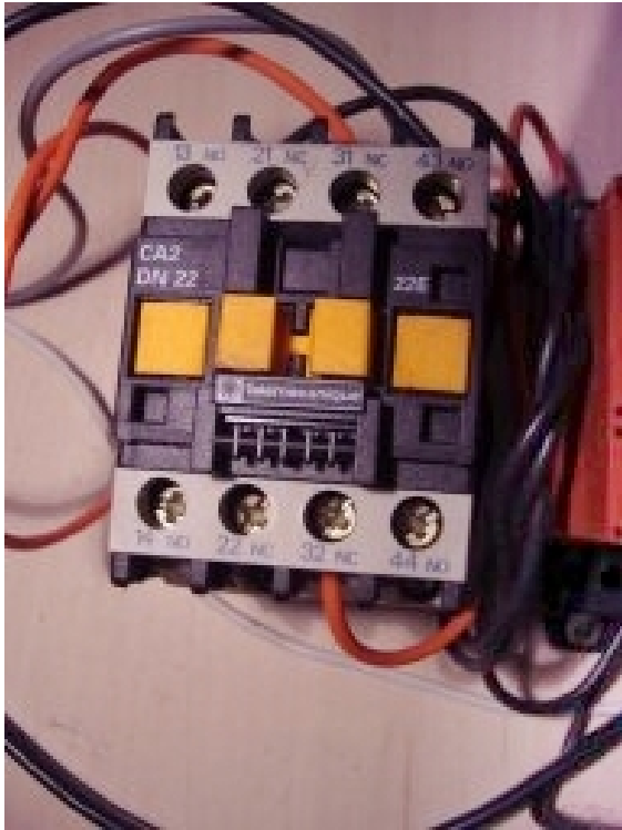
AC contactor for pump application.
