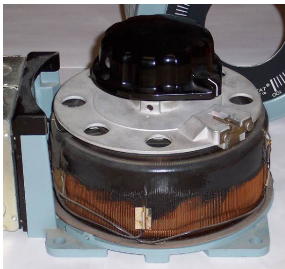
A variable autotransformer, with a sliding-brush secondary connection and a toroidal core. Cover has been removed to show copper windings and brush.
