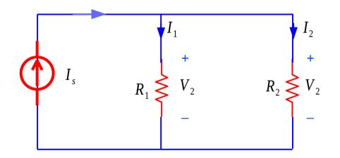
$$I_2 = \left(\frac{R_{eq}}{R_{eq} + R_2}\right) I_s$$
