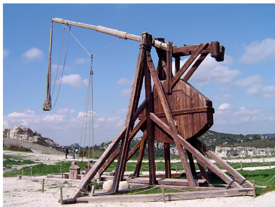
A trebuchet uses the gravitational potential energy of the counterweight to throw projectiles over two hundred meters
