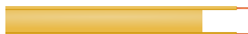
Fig. 4. Balanced line in twin lead format. This line is intended for use with RF circuits, particularly antennae.
