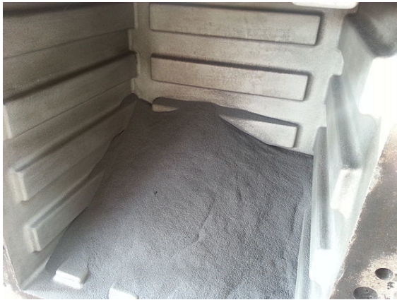
Raw material: XLPE powder used in Rotational molding in a factory.
