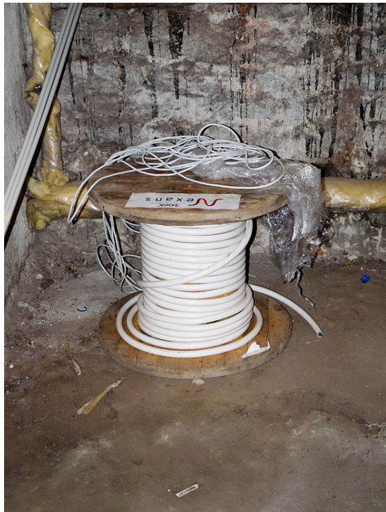
5 core PVC insulated copper cable
