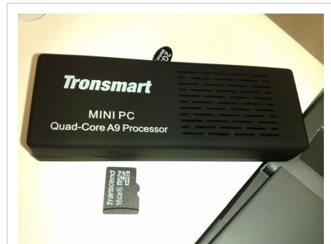
Tronsmart MK908, a Rockchip-based quad-core Android "mini PC", with a microSD card next to it for a size comparison.
