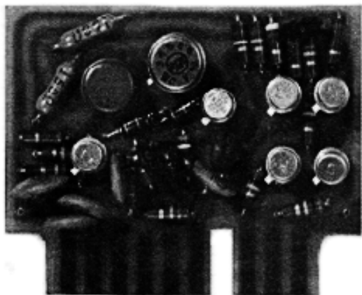
GAP/R’s model P45: a solid-state, discrete op-amp (1961).
