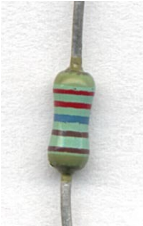
A 2260 ohm, 1% precision resistor with 5 color bands (E96 series), from top 2-2-6-1-1; the last two brown bands indicate the multiplier ( \times 10 ), and the 1% tolerance. The larger gap before the tolerance band is somewhat difficult to distinguish.
