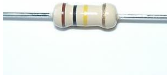
A 100 kΩ, 5% axial-lead resistor
