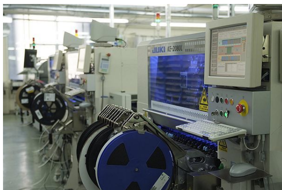
Assembly line with SMT placement machines
