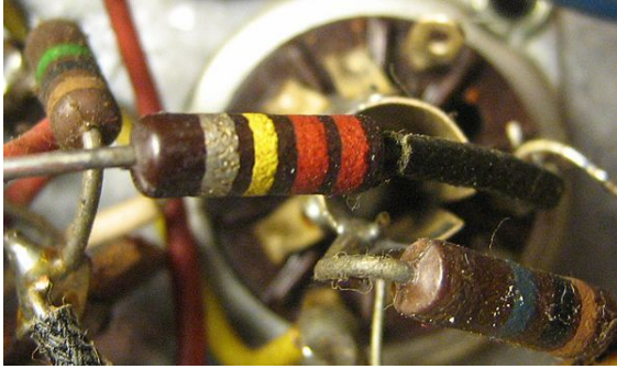
Three carbon composition resistors in a 1960s valve (vacuum tube) radio
