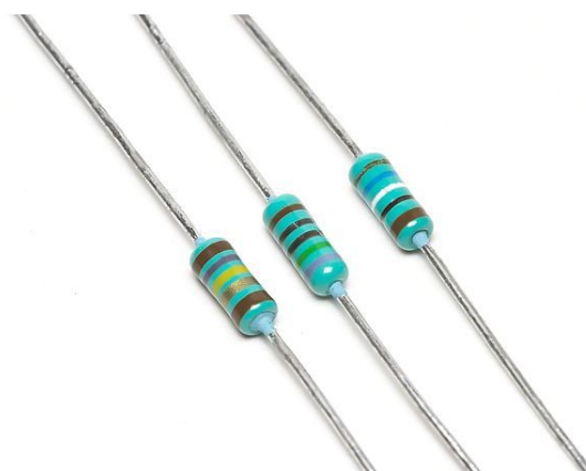
Resistors with wire leads for through-hole mounting
