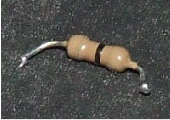
A 0 \Omega resistor, marked with a single black band
