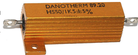
An aluminium-housed power resistor rated for 50 W when heat-sinked
