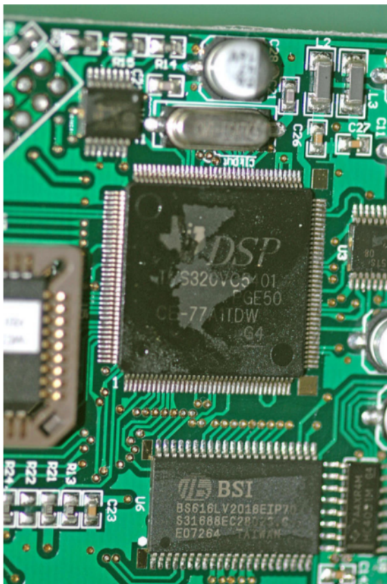
A digital signal processor chip found in a guitar effects unit.
