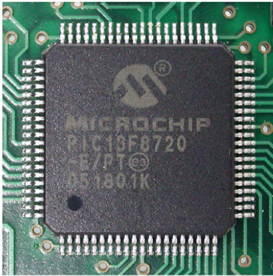
A PIC18F8720 microcontroller in an 80-pin TQFP package.
