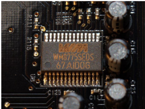
4-channel stereo multiplexed analog-to-digital converter WM8775SEDS made by Wolfson Microelectronics placed on an X-Fi Fatal1ty Pro sound card.
