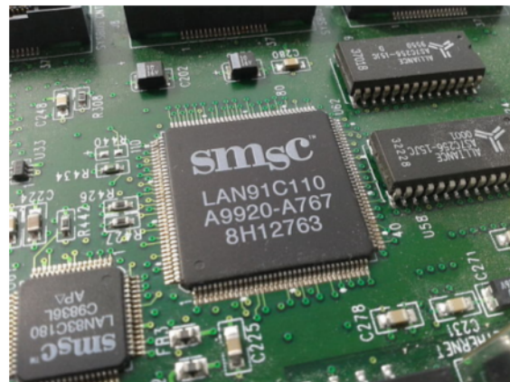
A close-up of the SMSC LAN91C110 (SMSC 91x) chip, an embedded ethernet chip.
