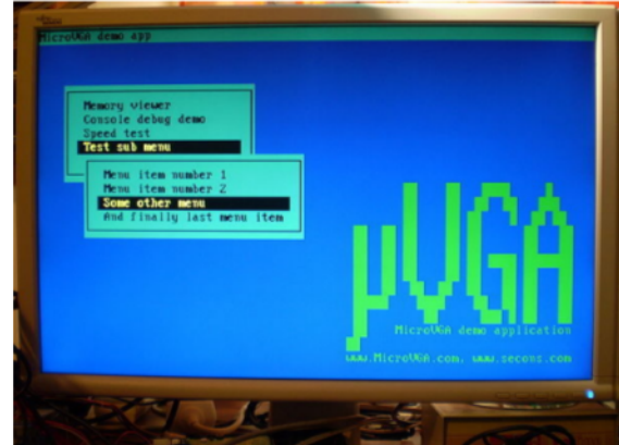
Embedded system text user interface using MicroVGA [nb 1]
