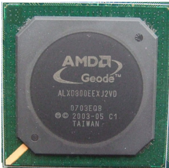
The AMD Geode is an x86 compatible system on a chip.
