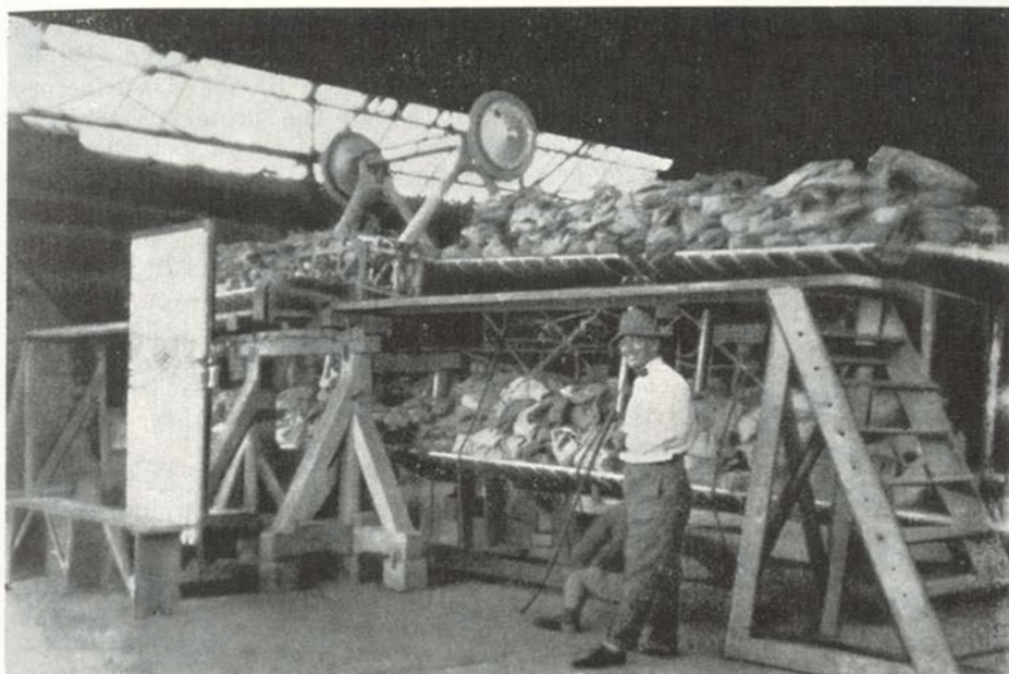
Static test of a Proto-2 plane, made in 1925 at the Astra factory of Arad.
